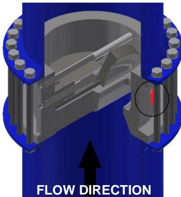
For mounting in pipeline the direction of the arrows that are located on the body should be equal to the flow direction.
